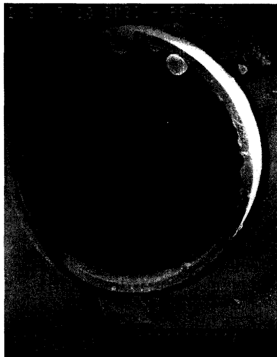
Fig. 10. EM of an imprinted CE capillary 10% (v/v) polymerizable groups in DMSO; ratio of the cross-linker to interactive monomer, 85:15; template, S (+)-2-phenylpropionic acid 5 mol.%; thickness of the coat, 4 μm; capillary diameter, 100 μm.
